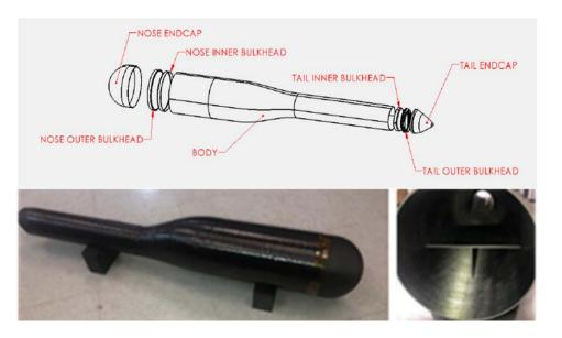
Figure 7. Tube-Launched UAS Test Platform (Source: H. R. Luzetsky).
