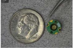
Figure 5. Radially Fired Laser (Source: S. Redington).
