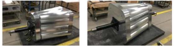
**Figure 7.** Breakaway Tool for Reinforced Fuselage Structure (Source: H. R. Luzetsky).
