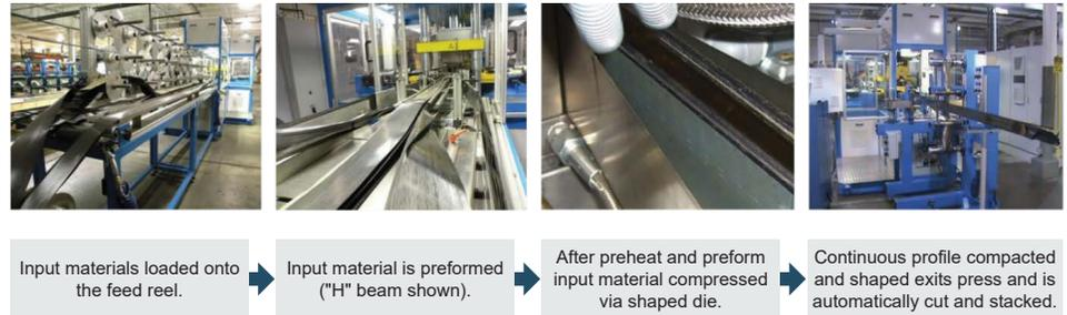
**Figure 10.** CCM Process Flow (Source: TSS/Albany).
