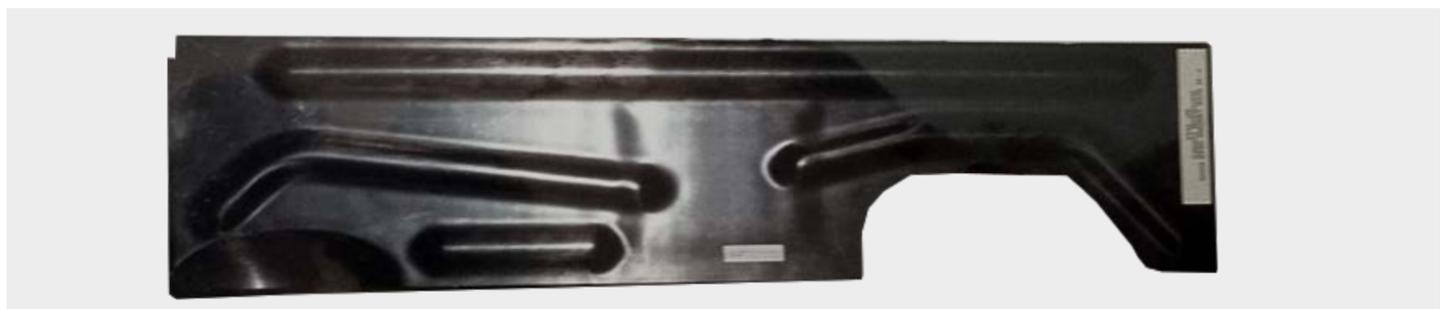
**Figure 3.** Prototype Landing Gear Door Formed From Double-Diaphragm Forming Process (Source: H. R. Luzetsky).
