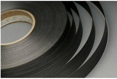
**Figure 6.** IM7/PEEK Thermoplastic Tape (Source: TSS/Albany).
