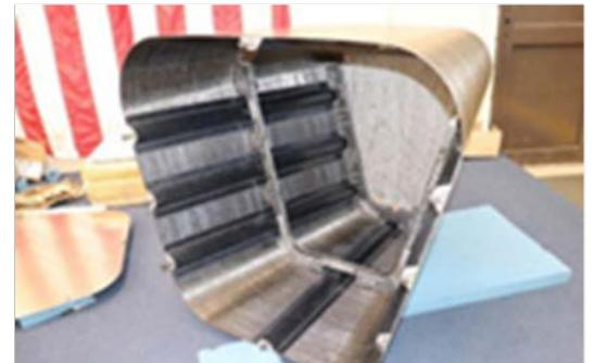
**Figure 8.** No-Fastener Assembly Structure (Source: H. R. Luzetsky).
