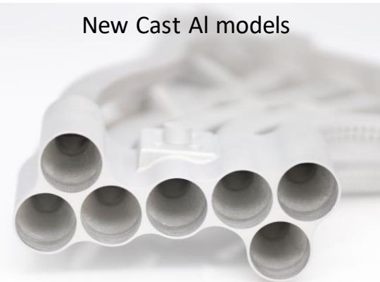
Cast Al models based on SLA mold
