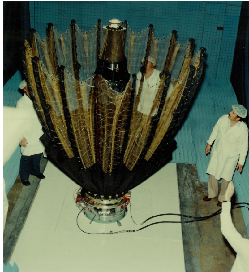
The Galileo antenna fully deployed (left) and partially deployed (above) while being tested on the plane polar nearfield antenna range at JPL's MESA Antenna Test Facility.
