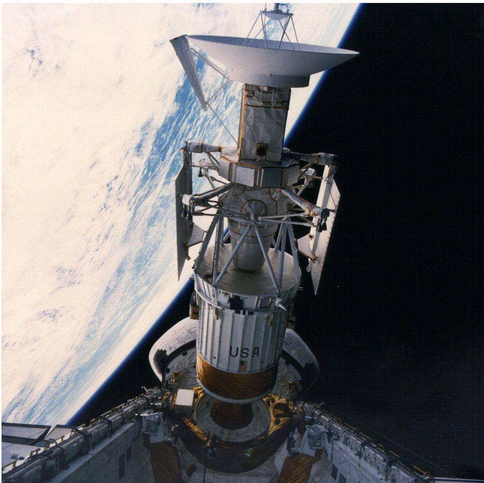
The Magellan spacecraft being deployed by the Space Shuttle Atlantis during STS-30, along with its inertial upper stage. To the left of the reflector antenna, the altimeter antenna instrument is also visible.
