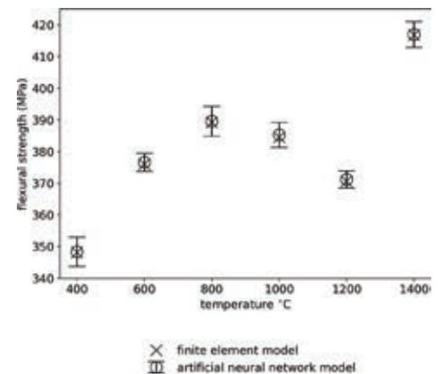
**Figure 6.** ANN and Physics Model Solved With FEM Prediction of FS vs. Temperature (Source: E. Walker, J. Sun, and J. Chen).
