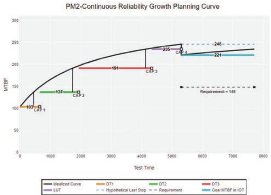
Figure 3. Example of Reliability Growth Planning Curve (Source: DAC).
