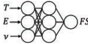
**Figure 2.** Inputs and Outputs of the ANN Surrogate Model (Source: E. Walker, J. Sun, and J. Chen).
