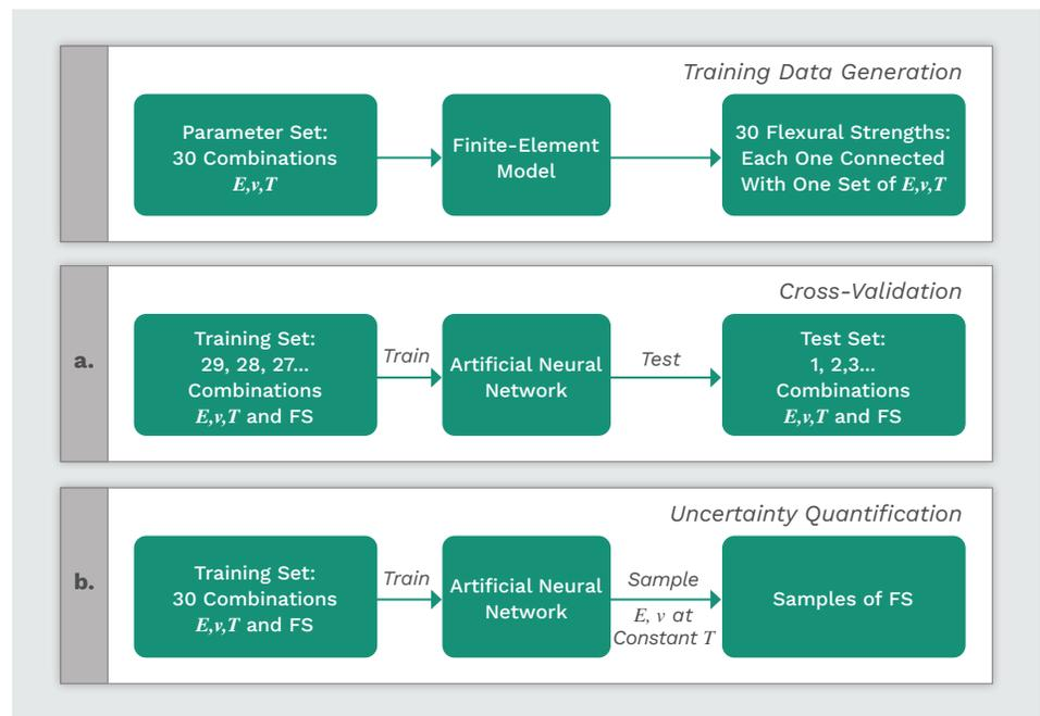
**Figure 3.** The FEM Training Data Set: (a) Cross-Validation for the ANN Reliability and (b) Forward UQ (Source: E. Walker, J. Sun, and J. Chen).
