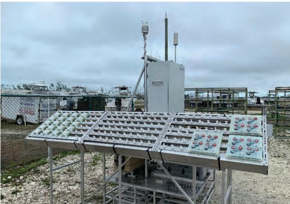
**Figure 3.** Instrumented Exposure Rack With Corrosion Test Coupons at NRL-Key West (Source: D. Hansen).
