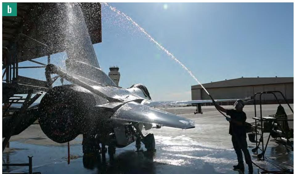
**Figure 1.** (a) Corrective Maintenance of Nonskid Coating on a Ship Deck (Source: U.S. DoD) and (b) Preventative Maintenance via Aircraft Rinsing (Source: U.S. Air Force).
