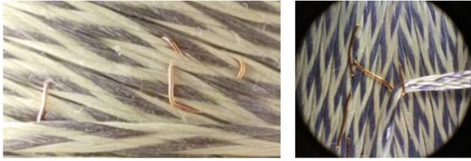
Figure 2-35. Tether Braking Hooks to Achieve Safe Payout Used on the TEPCE Cubesat Mission (Source: Coffey et al. [141]).
