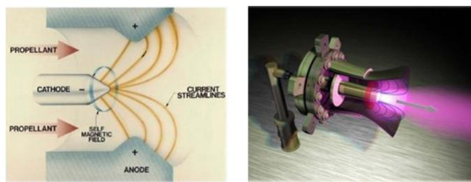
Figure 2-18. Diagrams of an MPD Electric Propulsion Engine (Source: NASA [69]).
