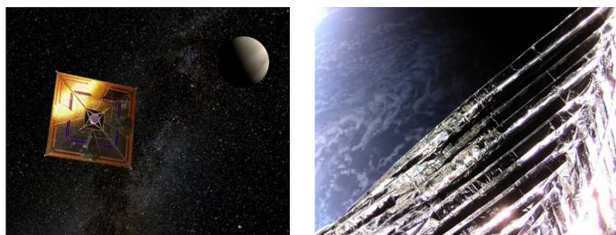
Figure 2-29. Publicity Image of the IKAROS Spacecraft (Left) and Image of the Deployed Sail on the ADEO Braking Sail Used for Deorbiting (Right) (Source: Wikimedia Foundation, Inc., [130] [Left] and ESA [131] [Right]).
