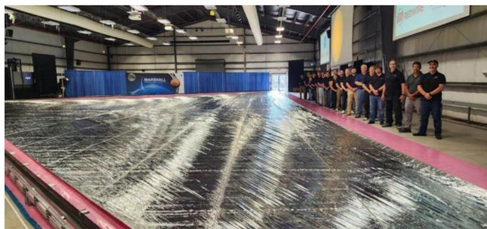
Figure 2-38. NASA's Solar Cruiser Sail (Made From a Flight-Proven Legacy Material—Thin-Film Polyimide [CP1] Coated With Aluminum) Unfurled to Show Its Size (Source: NASA [142]).
