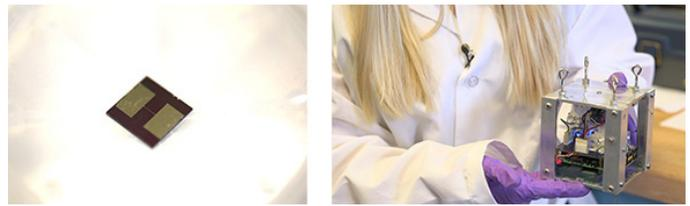
Figure 2-22. MEMS-Based Resistojet for CubeSats Using Steam (Source: Purdue University [78]).
