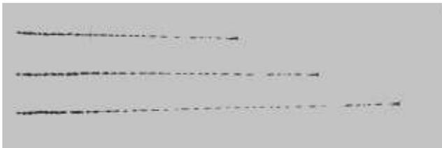
Figure 12-3. Radiograph of a Particulated Jet (Source: Dietrich [2]).
