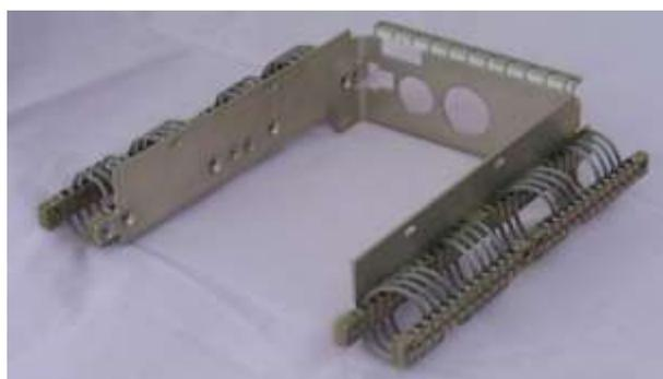
Four assemblies of coiled cables are captured between pairs of bars on the outside, two per side. This box mounted a hard disk drive.
