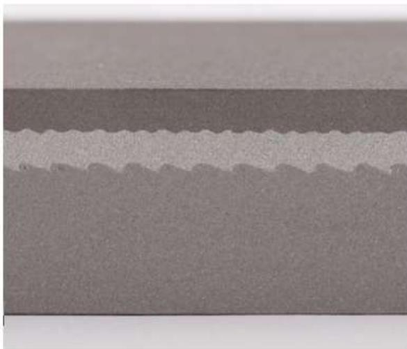
Three plates, explosively bonded. The cut is perpendicular to the collision line. The interlocking "breaking wave" patterns, similar to the familiar Greek stepped-fret motif, are caused by vortices forming and then being crushed together. Explosion welding can bond otherwise incompatible materials. Photo copyright and courtesy of NobelClad Co., Broomfield, CO. Used by permission.
