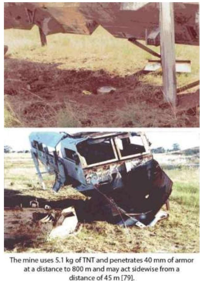
Figure 11-3. Casspir APC Hull Attacked by the TMRP-6 Antitank Mine (Source: Smit [80], Used by permission).
