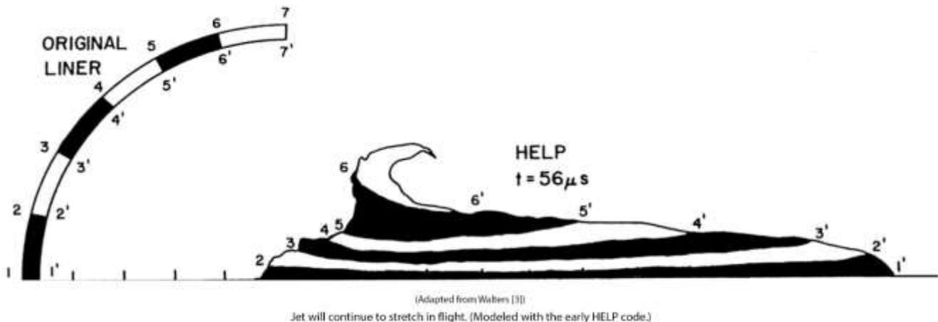
Figure 2-7. Penetrator from SC with Hemispherical Liner (Source: Dietrich [2]).
