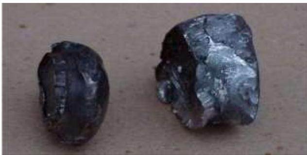
Figure 5-4. Residual Penetrator (left) and Target Plug (right) (Source: Silsby [1]).
