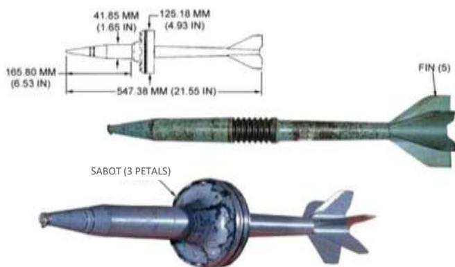
U.S. Navy EOD graphic. Nose has been damaged. Not clear are canted holes in the three sabot petals that impart spin as gun gases are vented up the bore, copper buttons on the substantial steel fins that act as bore riders, and machined leading edges on the fins that create lift to lock the round into a desired roll rate in flight.
