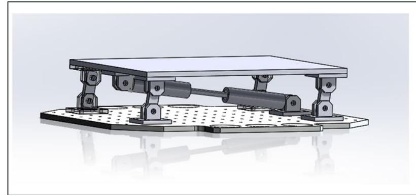
Vertically oriented four-bar fixture
