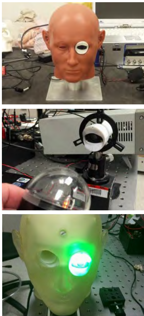
Figure 8: Eye Sensor Mounted in Surrogate (Top), Benchtop Mount (Middle), and Exposed to Green Laser Light (Bottom) (Source: CFDR).
