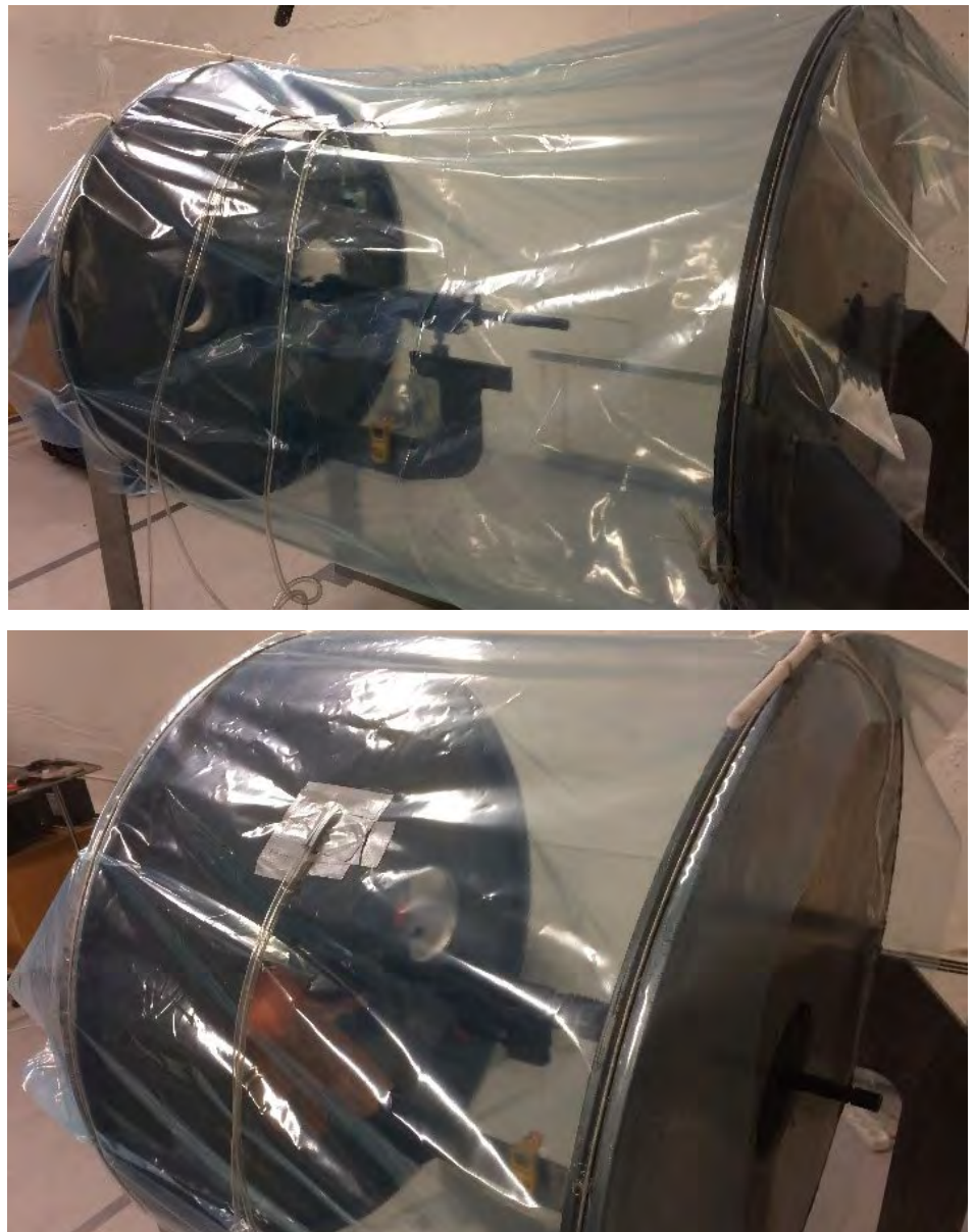
Figure 1: Chamber With Weapon Muzzle Inside (Total Propellant Gas, Top) and Muzzle Outside (Blowback Gas Only, Bottom) (Source: Norwegian Defence Research Establishment [FFI]).
