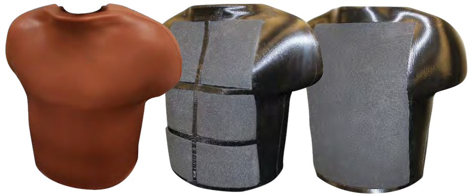
Figure 6: Blunt Torso (Left), Six-Pad EM Torso (Middle), and Single-Pad EM Torso (Right) (Source: CFDR).
