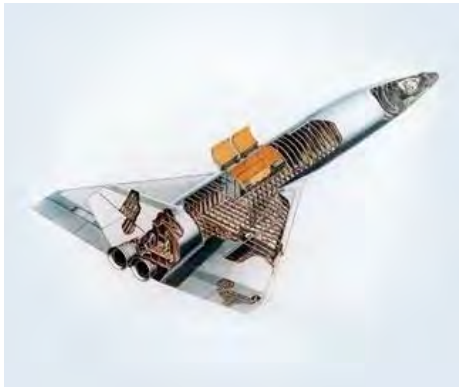
Figure 9: Boeing's Late 1970s Design of the Reusable Aerodynamic Space Vehicle (RASV) (Source: Boeing).
