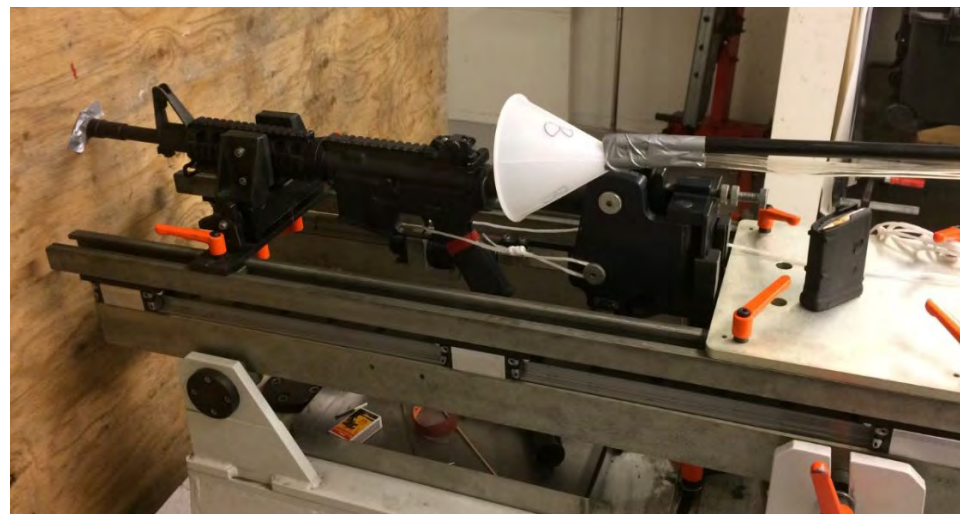
Figure 2: Weapon and Sampling Setup for the Breathing Zone Test Method, Left Inlet (Source: FFI).
