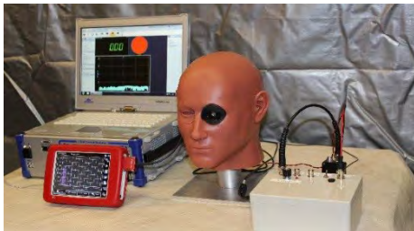
Figure 12: Surrogate Head Evaluation With Sound, Pressure, and Ocular Sensors Using Concurrent Data Collection (Source: CFDR).
