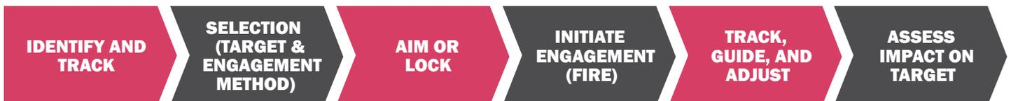
Figure 1: Fire Control Kill Chain (Source: ARDEC).
