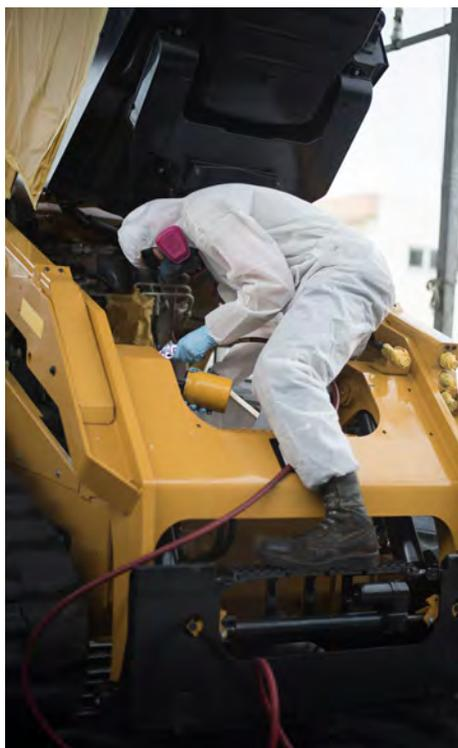
Figure 3: Spraying Coatings Inside Engine Compartment to Provide Extra Protection Against the Corrosive Environment (Source: Senior Airman Omari Bernard, 18<sup>th</sup> Wing Public Affairs).
