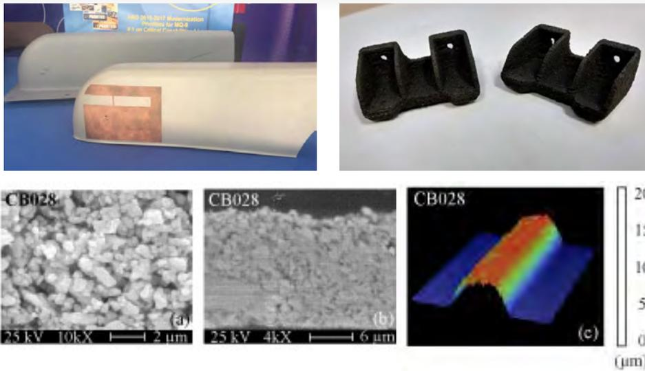
Figure 9: Examples of USAF AM Technologies for Functional and Extreme Environments: Direct-Write Plasma Technology to “Print” a Cu Antenna on an MQ-9 Reaper (Top Left), Printed High-Temperature Carbon Fiber Composite (Top Right), and Images of Silver Ink Used to Print Resilient Hybrid Electronics Onto PEEK (Bottom) (Sources: Pawlyk, Neff et al., and AFRL [18-20]).
