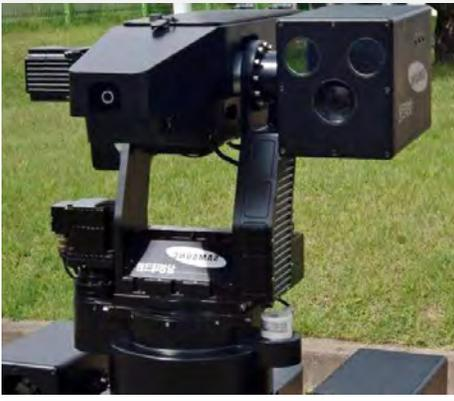
Figure 5: SRG-A1 Autonomous Weapon (Source: SGR-A1 [12]).
