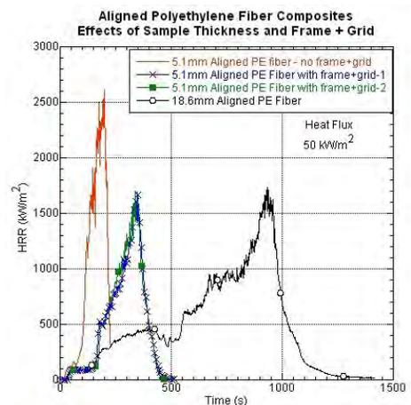
Figure 3: HRR Curves for Phenolic + S-2 Glass FRP Spall Liners (Top) and Ultrahigh Molecular Weight Polyethylene Spall Liners (Bottom) (Source: Morgan [6]).
