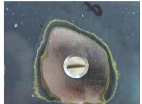
Figure 5: Example of Cold Spray Repair of B-1 Bomber Aircraft FEB Panel Showing Chafing Wear on Fastener Hole (Left) and Then After Grit Blasting, Cold Spray Repair, Grinding, Polishing, and Final Hole Machining (Right) (Source: Widener [13]).
