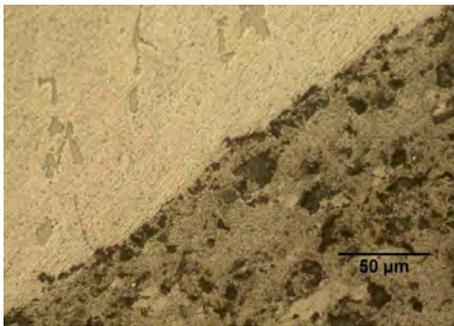
Figure 6: Strong Interface Between Cold Spray and Original Material (Source: Widener [13]).
