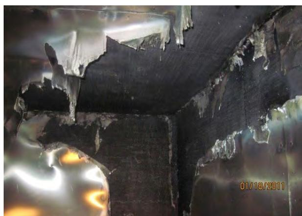
Figure 5: Example of Fire Protection Barriers – Ceramic Fiber Blankets (Left) and Metal Skins Enabling Composites to Pass the Room Corner Test (Right) (Source: Morgan and Toubia [11]).
