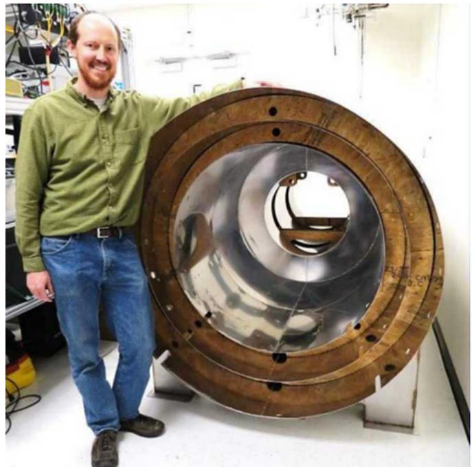
Figure 5-1. Mu-Metal Enclosures Used to Create EM Shielded Areas [65].
