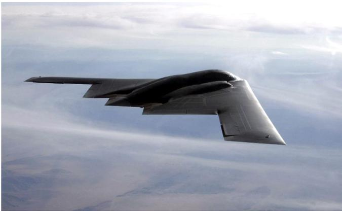
Figure 2-3. The B-2 Bomber With Radar Absorbing Coating and Characteristic Radar Minimizing Geometry (Source: <https://www.af.mil/About-Us/Fact-Sheets/Display/Article/104482/b-2-spirit/>).
