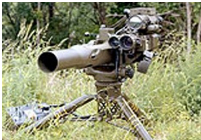
Figure 6-3. TI Common Module FLIR-equipped TOW sight (Source: TI).
