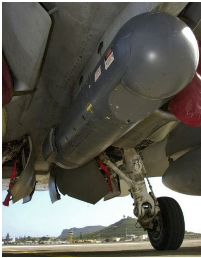
Figure 10-4. The U.S. Air Force LITENING G4 pod uses active imaging for extended-range target identification (Source: USAF).
