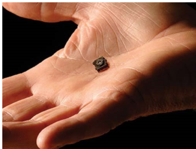
Figure 10-2. The Lepton microbolometer is an example of how small IR imaging sensors can be made. They can be used for covert, unattended operation in either remote or urban locations and connected to the battlefield network (Source: FLIR Inc.).
