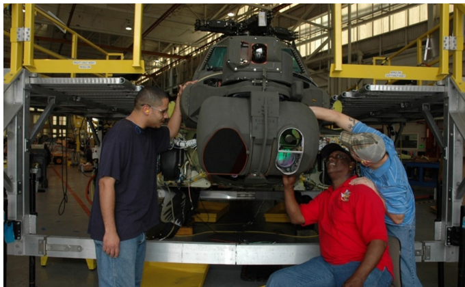
Figure 1-5. Apache attack helicopter Modern Target Acquisition and Designation Sight (MTADS) targeting system (Source: U.S. Army Photo/Brigitte Rodriguez).
