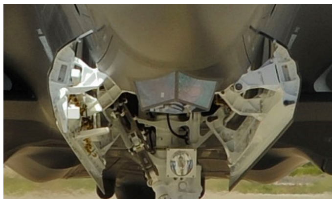
Figure 8-8. F35 Distributed Aperture Sensor (DAS) employed multiple staring InSb-based FPAs. Larger-format arrays provided enhanced target acquisition range allowing weapons platforms to engage from the relative safety of higher altitudes (Source: U.S. Air Force).
