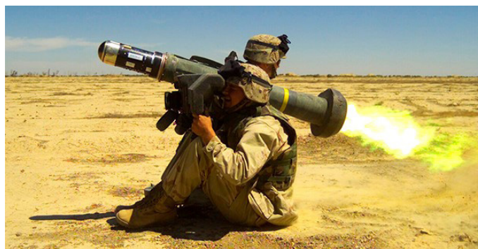
Figure 8-3. The Javelin antiarmor missile has a staring seeker 64x64 LWIR FPA from Raytheon Vision Systems (RVS [HAC]) in the missile and a scanning sensor with a linear LWIR FPA from DRS (TI) in the command launch unit. The target is acquired with the command launch unit FLIR, which relays that information to the seeker, which tracks the target and determines the point of impact (Source: U.S. Army).
