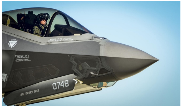
Figure 1-7. F-35 with IRST and Missile Warning Receiver (MWR) Distributed Aperture Sensor (DAS) (Source: U.S. Air Force photo/Senior Airman Christopher Callaway).
