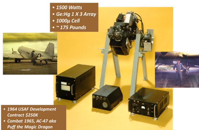
Figure 5-1. First flyable FLIR made by TI. It was the first FLIR to be tested on an AC-47 gunship (1965). Right inset shows Kirby Taylor standing beside the gunship at Bien Hoa Air Base, Vietnam (Photo Credit: Kirby Taylor [21]).
