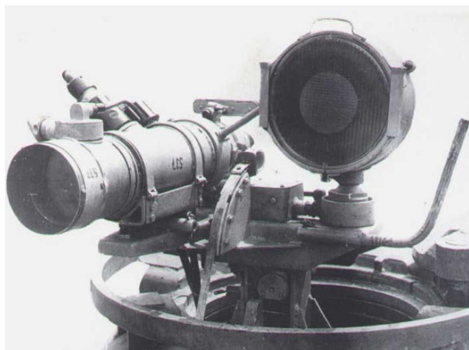
Figure 3-3. German Panzer FG 1250 searchlight and scope (Source: Williams [17]).
