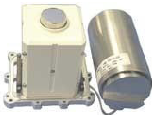
Figure 8-6. The principal GEN2 Common Module IDCA (Integrated Detector Dewar Assembly), (left), contained a 480x4 LWIR MCT FPA, (right), in a sealed Dewar with cryocooler and drive electronics. The additional pixels on target and TDI feature provided a significant range advantage over GEN1 imagers (Source: Laser Focus World [left photo] and Opto-Electronics Review [right photo]) [50].
