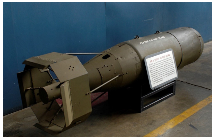
Figure 3-4. U.S. VB-6 IR guided bomb (Source: USAF).
