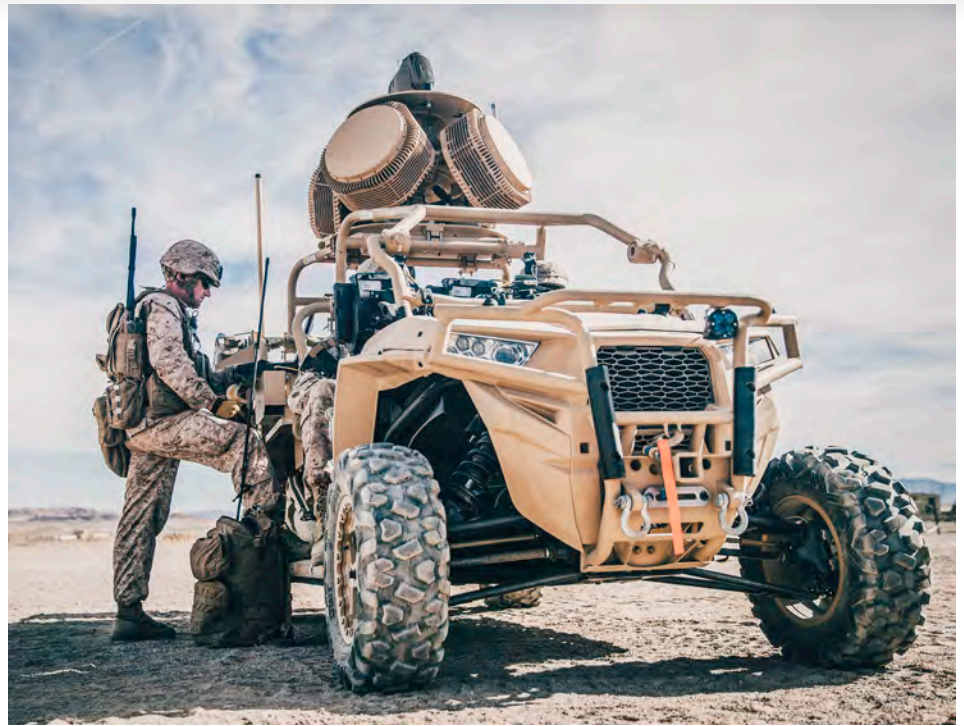
Figure 4: L-MADIS Light Marine Air Defense Integrated System (Source: PM GBAD, USMC [25]).
