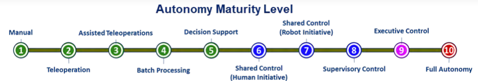
Figure 4: Autonomous Behavior Characteristics for Independent Operation (Source: Lockheed Martin).
