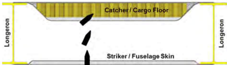
Figure 1: Turning Block Spaced Armor Integrated With Aircraft Skin and Floor Sections (Source: Robeson [2]).
