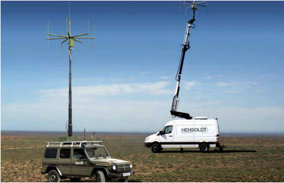
Figure 5: Commercial PCL Radar Example (Source: Hensoldt [3]).
