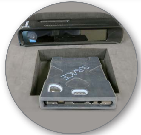
Figure 7: Hawkeye Scanner With Battery Pack.
