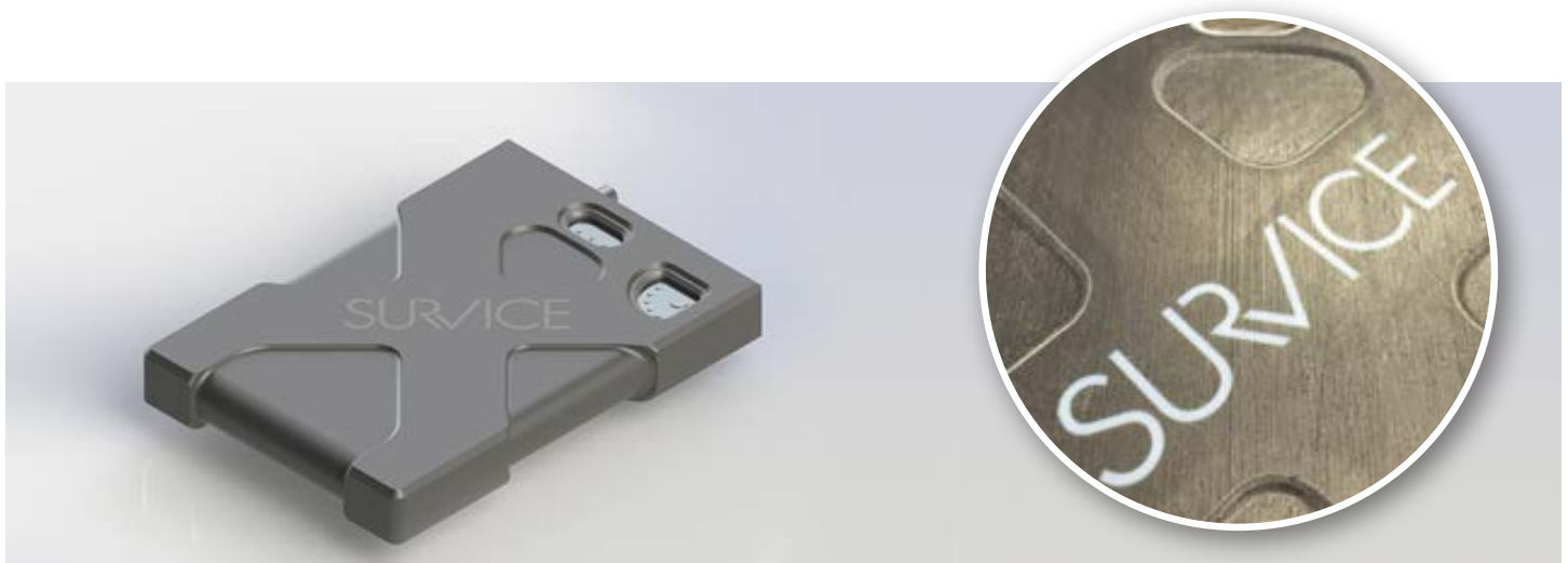
Figure 9: Hawkeye Rendered Battery Pack Case Model (left) and Polyjet-Printed Two-Material Battery Case (right).
