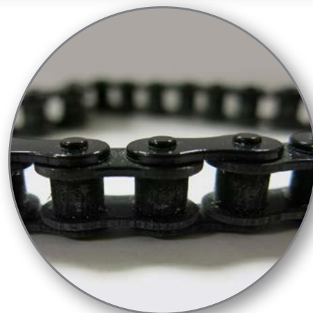
Figure 5: Assembled Chain Printed With Polyjet Technology.
