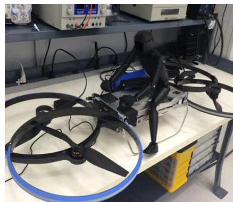
Figure 11: FDM-Printed Components on Hoverbike Scale Model.
