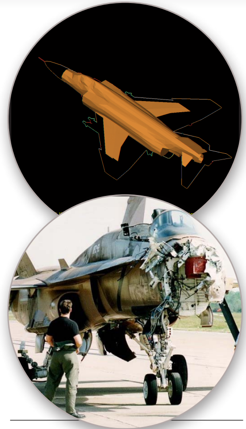
Figure 1 (top): Colored Surfaces Indicating Regions of Example Aircraft Vulnerable to Blast and Direct Kills.
