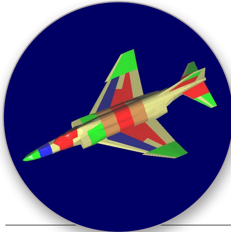
Figure 7: Example of MSPK Output for a Specific Fragment Mass, Speed, and Attack Direction. In Practice, the Skin Would Be Divided Into Tens to Hundreds of Components, and the Pk Values and Color Would Change as the Mass, Speed, or Attack Direction Changes.
