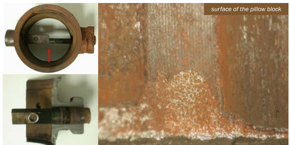
Figure 6: Engine Break Butterfly Shaft Seized Inside Iron Pillow Block [2].
