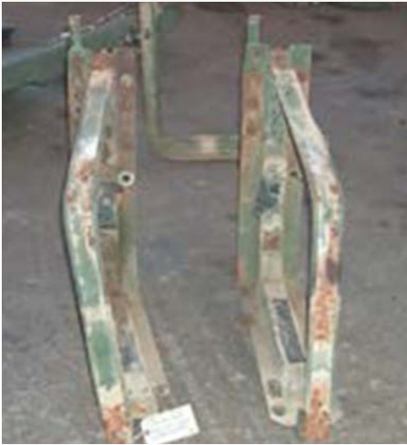
Figure 11: MTRV Corroded Fuel Tank Straps [2].
