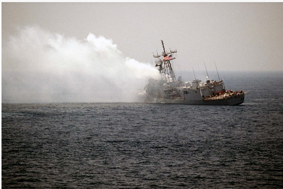
Figure 1: Damage to the USS Stark From Two Antiship Missile Hits (Source: U.S. Navy).
