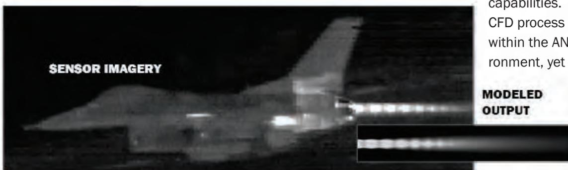
Figure 6: Measurement Sensor Image Compared to High-Fidelity QF-16 Modeling Process Output.
