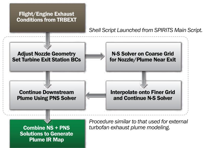
Figure 2: Insertion of High-Fidelity QF-16 Plume Modeling Methodology into Legacy DoD Process.
