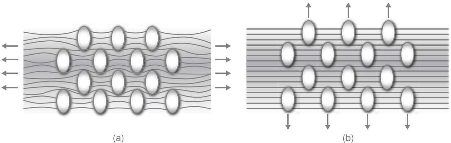
Figure 4: Nodule/Fibril Structure. (a) Slack Fibril/Nodule Structure with Direction of Stretch Illustrated. (b) Stretched Fibril/Nodule Structure with Direction of Expansion Marked.
