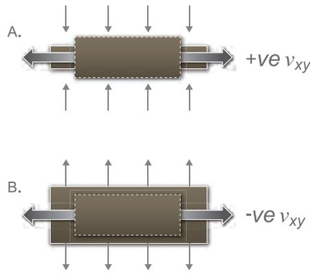
Figure 1: Illustration of Deformation for (A) Positive Poisson's Ratio Materials, (B) Negative Poisson's Ratio Materials.<sup>5</sup> Image Reproduced From Auxetnet Website.
