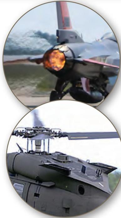
Figure 1: QF-16 Exhaust Nozzle (top [2014© William Schenck]) and UH-60M with UES Aft of Main Rotor Hub (bottom).
