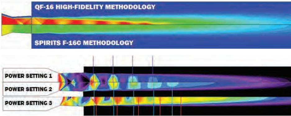
Figure 4 (top): Comparison of Flowfields as Generated by Legacy Process and Modified Legacy Process. Figure 5 (bottom): Generic H-60M Process Used to Determine QF-16 Shock Diamond Centroid Locations Across Three Power Settings.
