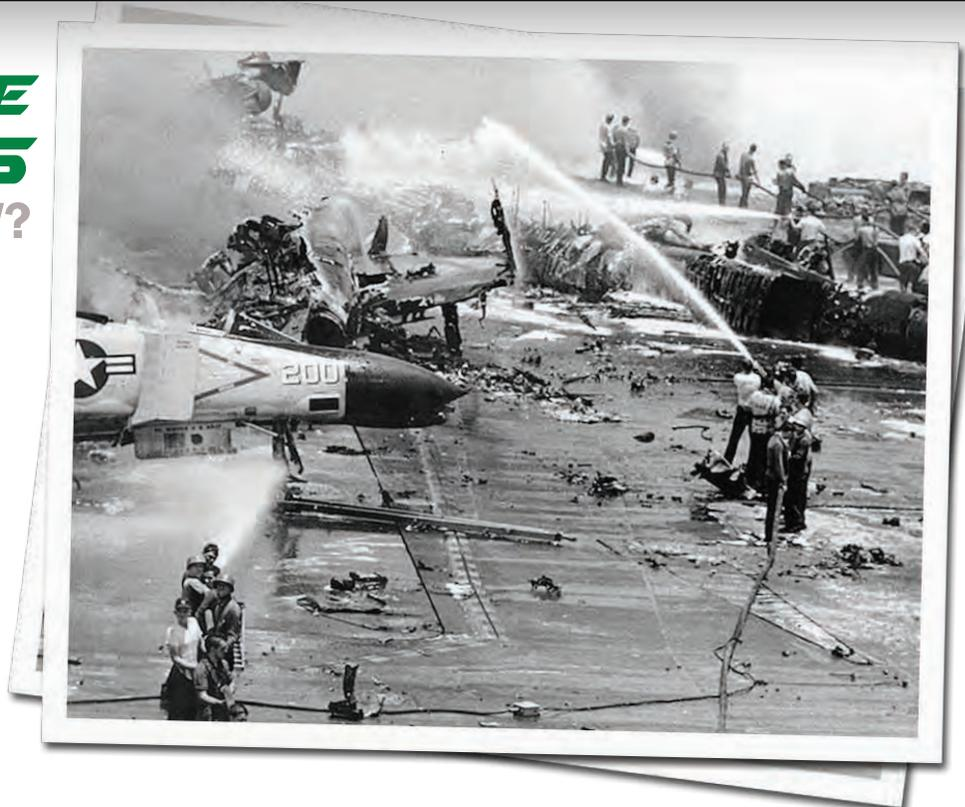
Figure 1: USS *Forrestal* Aircraft Carrier Fire Caused by Weapon Cookoff.
