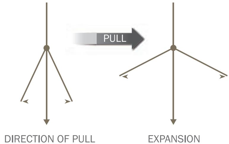
Figure 2: Basic Deformation Mechanism for Auxetic Materials. An Applied Tension in the Vertical Direction Causes the “Opening” of the Arms, Resulting in Expansion in the Direction Perpendicular to the Force.
