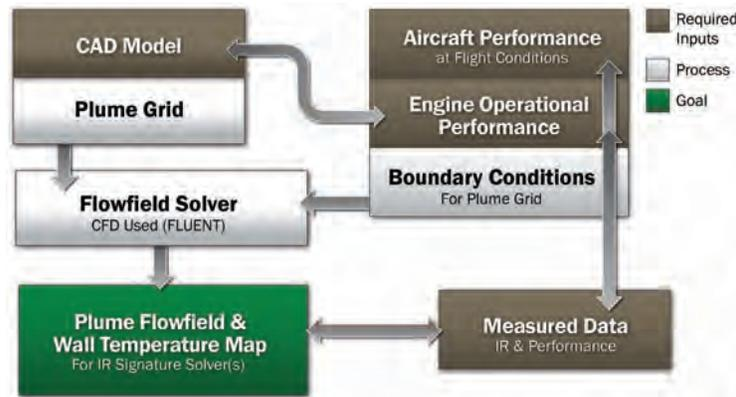
Figure 3: Generic CFD-Based Process as Used in H-60M Plume Modeling.
