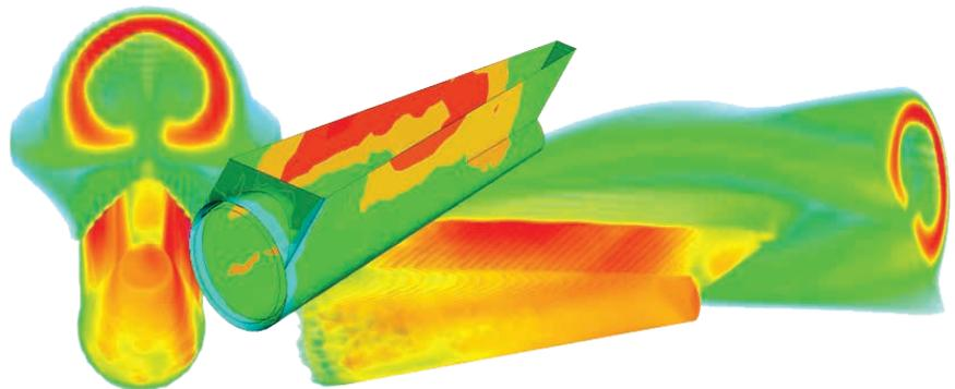
Figure 8: CFD Based Flow and Wall Temperature Mapping for a Notional Turboshaft Mixer-Ejector Exhaust System.
