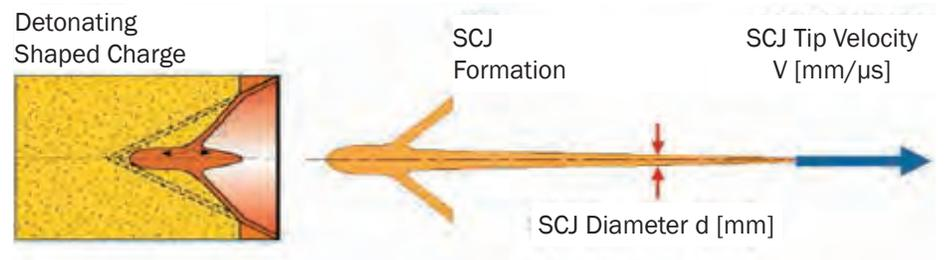
Figure 2: Illustration Of Shaped Charge Jet Diameter ( $d$ ) and Velocity ( $V$ ).<sup>5</sup>
