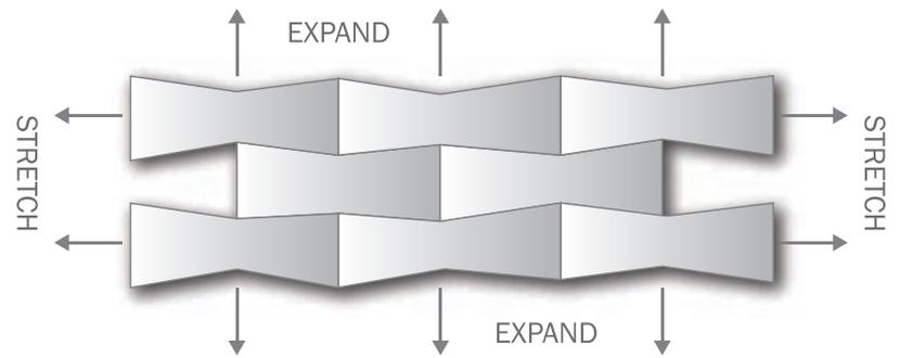
Figure 3: Basic Re-Entrant Network Structure. As the Structure Is Stretched Horizontally, the “Bow-Tie” Structures Open Vertically, Resulting in Expansion in the Direction Perpendicular to the Force.
