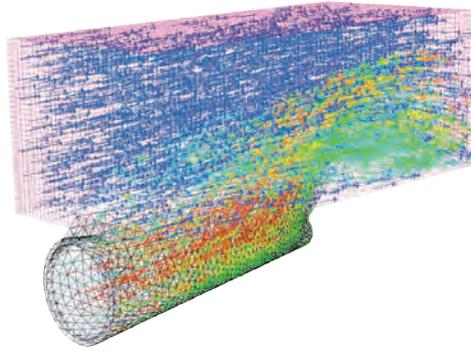
Figure 7: Flow Velocity Vectors and Temperature Visualized on Top of a Predominately Auto-Generated Mesh.
