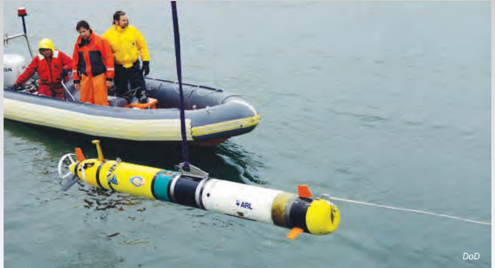
Figure 2: REMUS 600 AUV, Used to Map Sea Floor with Sonar Sensors.
