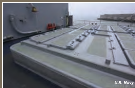
Figure 4: Removed VLS Crane.
