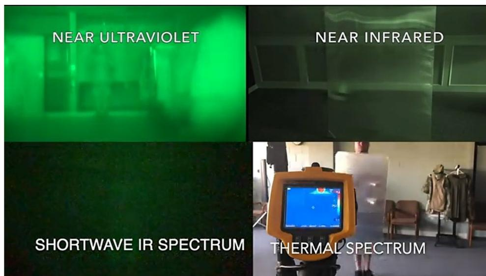
**Figure 12: Quantum Stealth Material Demonstrated Obscuring Person in Various Spectral Bands [31].**
