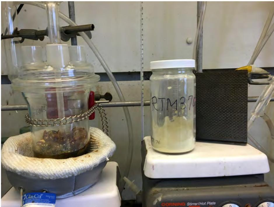
Figure 2: Synthesis of a Crosslinkable Polyimide (Source: AFRL).
