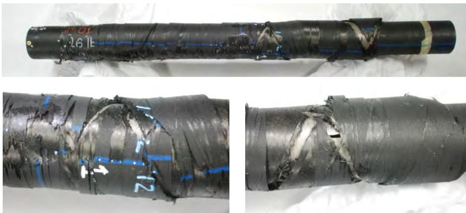
Figure 5: Failed Composite Tube (Source: CCDC AC).
