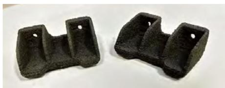
Figure 7: Reduced Scale (0.5x), Selective Laser-Sintered Brackets With High Service Temperature Capabilities (300 °C) (Source: AFRL).
