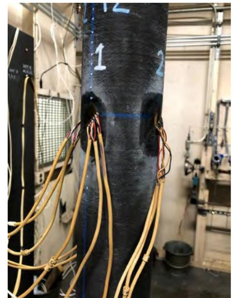
Figure 4: Tube in the Hydraulic Press (Left) and Close-up of Strain Gage Location (Right) (Source: CCDC AC).
