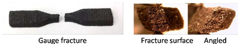
Figure 6: Images of a Fractured Specimen After Tensile Testing (Source: AFRL).
