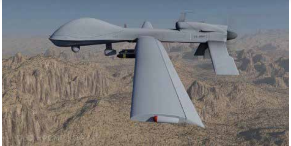
Figure 1: Rendered Army Gray Eagle MQ-1C Powered by a Turbocharged 160-hp Diesel Engine (Source: DoD).
