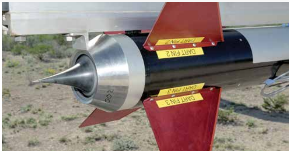
Figure 7: Close-up Photograph of Blacksky's Aerospike Nozzle Flown in 2004 (Source: NASA).
