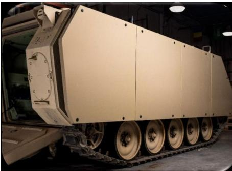
Figure 10: Prototype ARDDM Kit Integrated Onto M113 Troop Carrier (Source: QNA).
