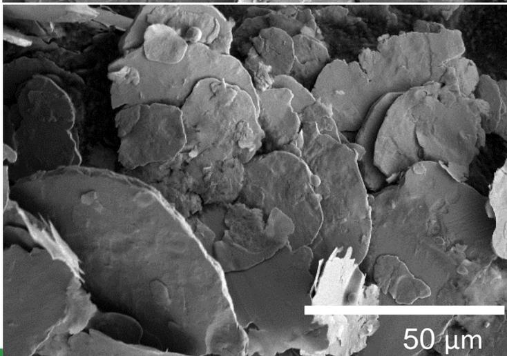
Cryomilled, Degassed, and Sieved (-325 Mesh)
