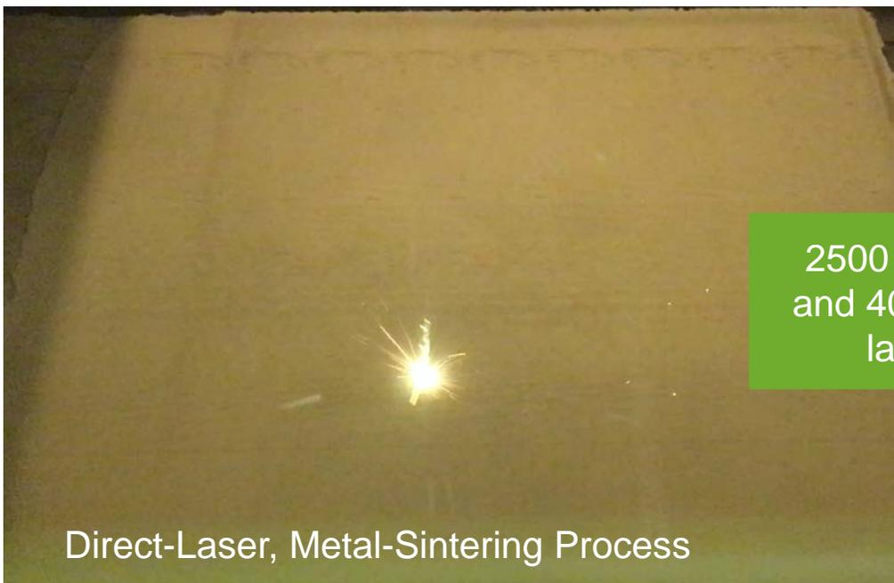
Direct-Laser, Metal-Sintering Process
