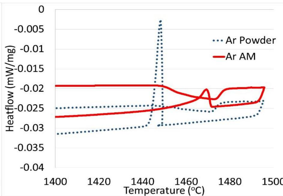
Cryomilled Powder Melting: 1463-1476 °C
