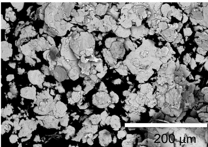
Cryomilled, Degassed, and Sieved (-325 Mesh)
