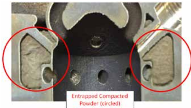
Figure 6-1. A cutaway of an AM part with trapped impacted powder (circled in red) that would be impossible to remove postbuild (30).
