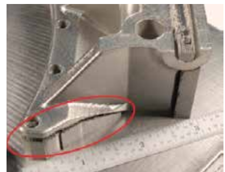
Figure 1-8. Cracking and delamination can result from residual stresses in the part during the build process (11).
