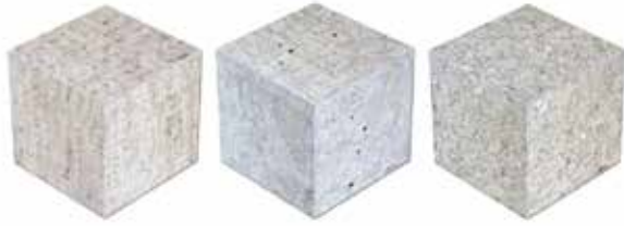
Figure 6-2. (Left) An as-built cube of material; (middle) the same cube after undergoing stress relief; (right) the same cube after undergoing HIP and final machining (31).
