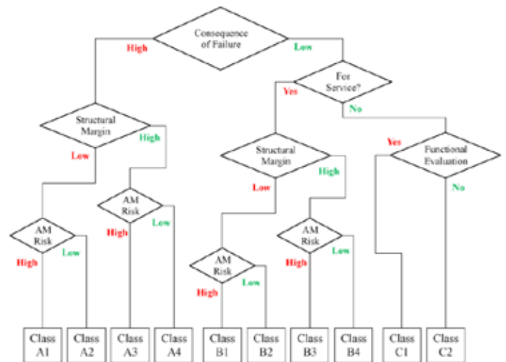
Figure 13-2. The AM certification risk schedule helps sort the parts into risks groups to guide the customization process (40).
