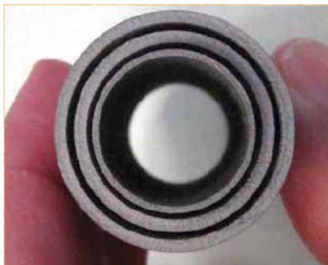
Figure 1-1. Titanium “tube in a tube” for a cryothermal switch on the ASTRO-H satellite. Traditional manufacturing would cost up to $20,000 and take 3 months to build. AM can drop the cost to $1,200 and the wait time to 2 weeks (5).
