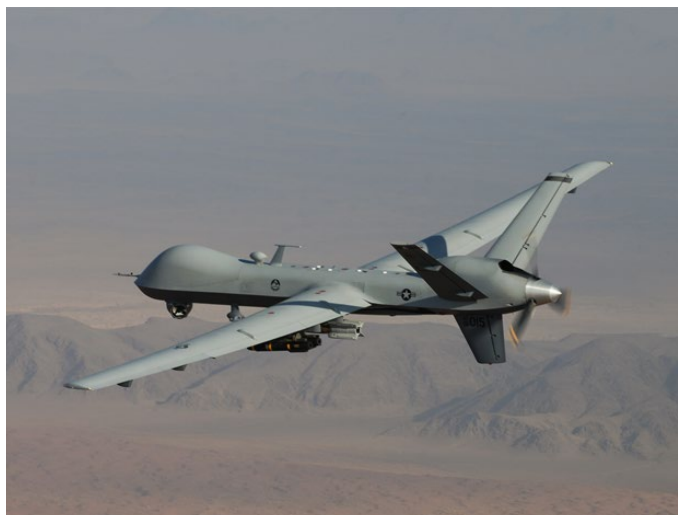
Figure 6-3. The MQ-9 Reaper is larger and more heavily armed than the MQ-1 Predator and is used for attack and IRS missions (Source: U.S. Air Force Photo / Lt. Col. Leslie Pratt).
