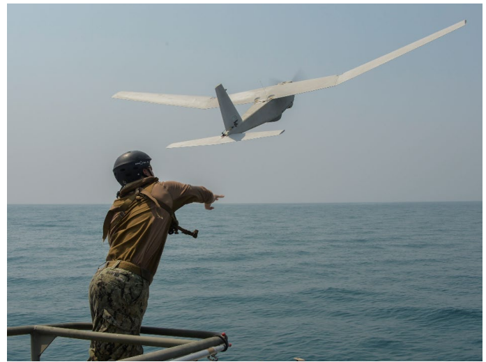
Figure 6-5. A Puma AE UAS is hand-launched from a Riverine Command Boat (RCB) at sea (Source: U.S. Navy photo by Mass Communication Specialist 1st Class Peter Lewis).
