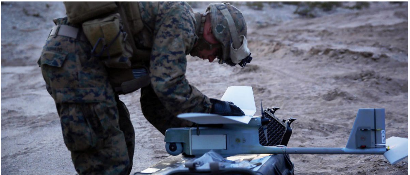
Figure 6-1. The Raven is a self-contained, rucksack-portable UAS that is remotely operated and used in support of combat battalion-level and below operations and other combat support units (Source: U.S. Marine Corps).
