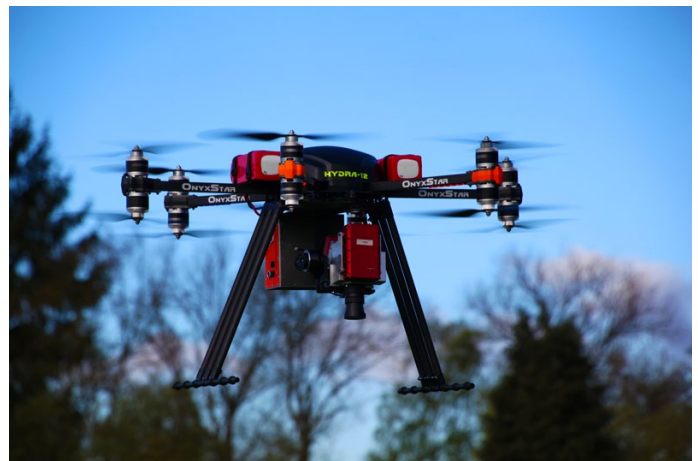
Figure 7-1. Onyxstar HYDRA-12 UAV with embedded hyperspectral camera for agricultural research (Source: Cargyrak [CC BY-SA 4.0], from Wikimedia Commons).
