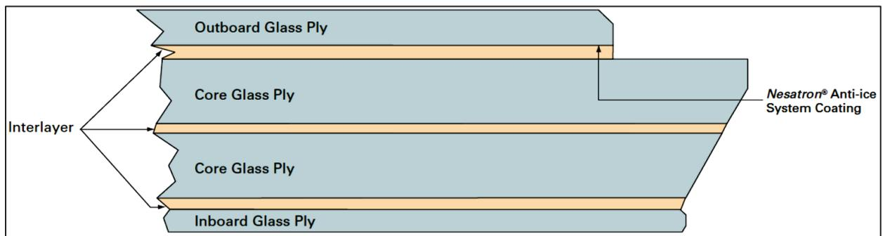
**Figure 9: A-10 Center Windshield (Glass Plies, Urethane Interlayers) [14].**
